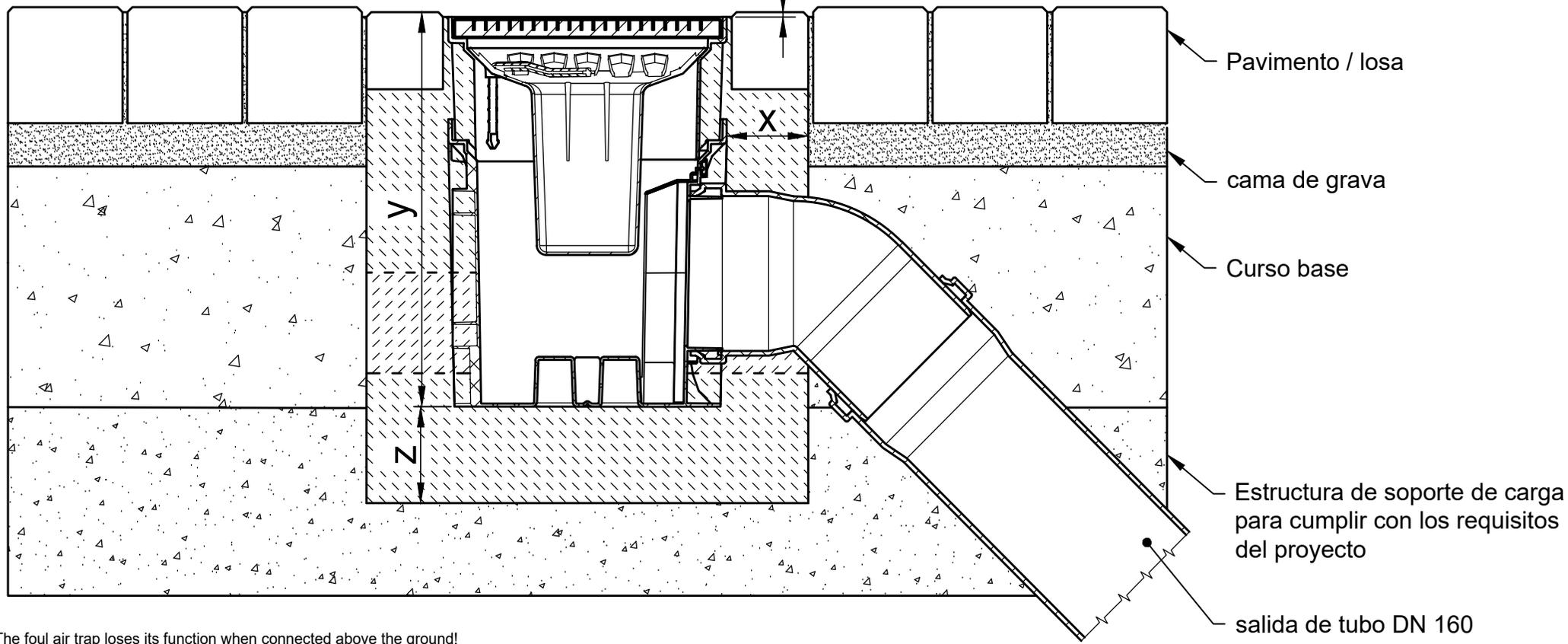
Attention: The foul air trap loses its function when connected above the ground!
